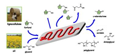
**Scheme 1.** Continuous catalytic production of biosourced chemicals from furfural, glycerol and analogues via different intermediates.
